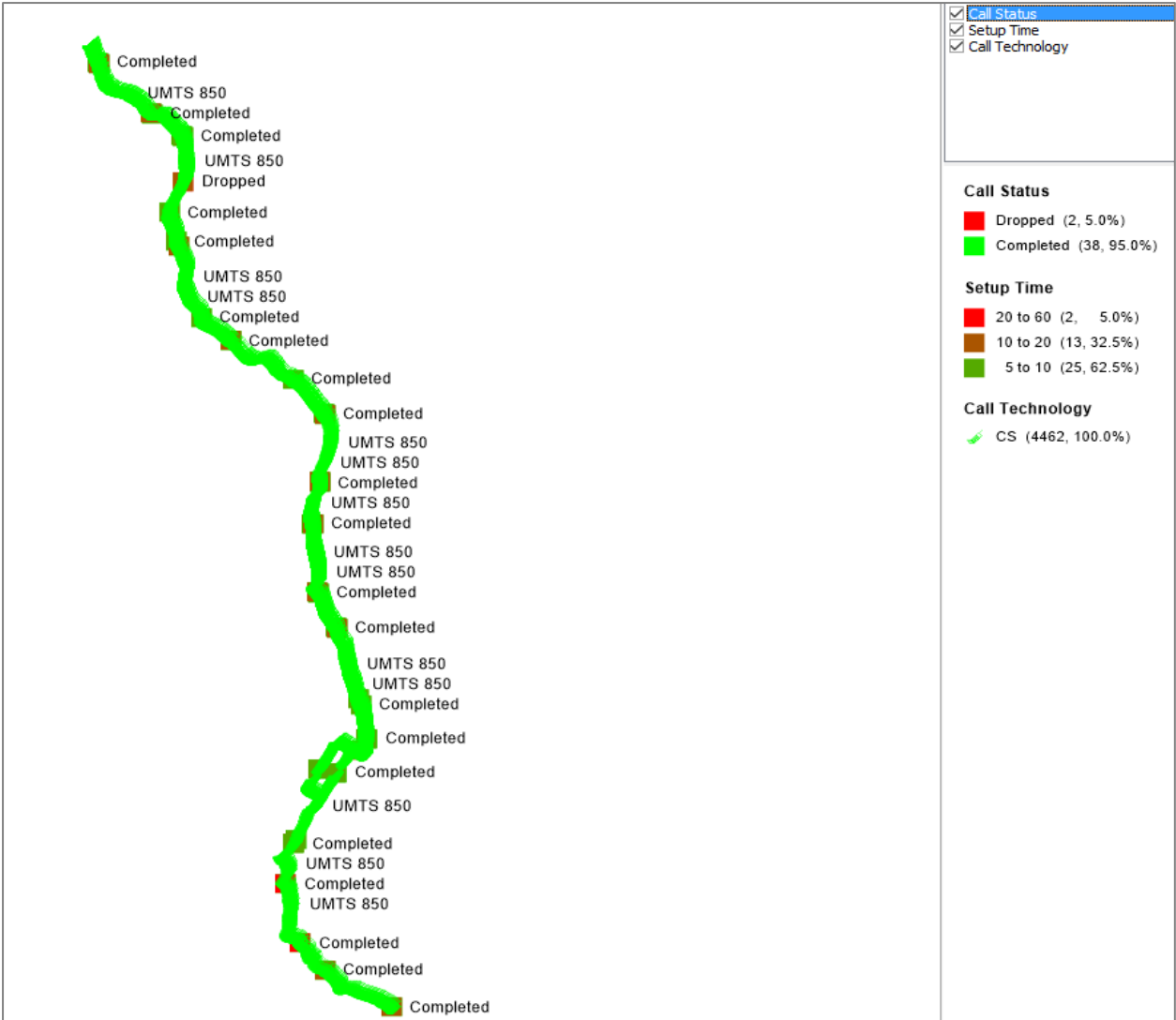
Figure 17: Map of Call Set-Up Time, Call Status and Call Technology of Bmobile and TashiCell for 3G Network(Punakha)
