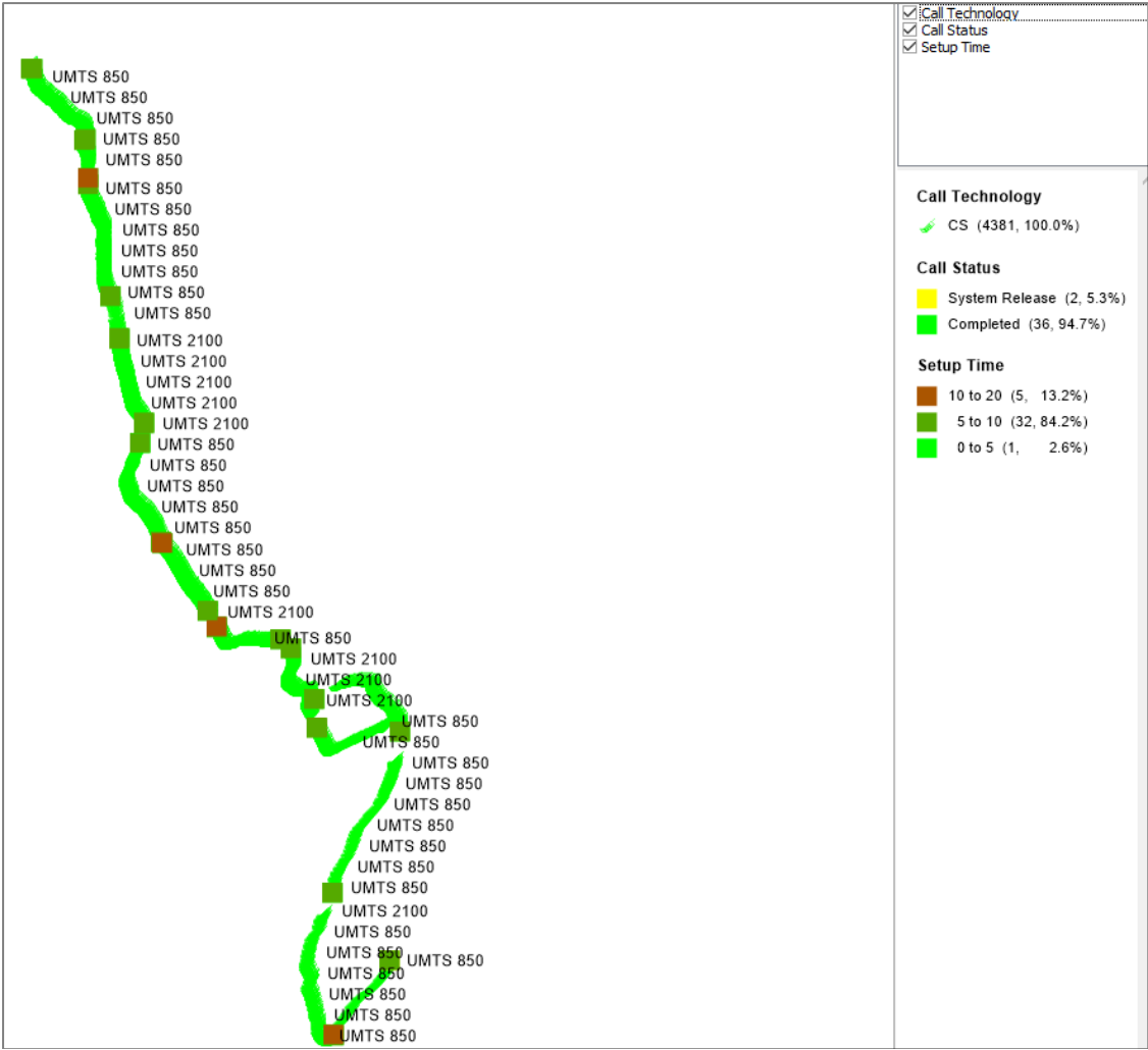
Figure 13: Map of Call Set-Up Time, Call Status and Call Technology of Bmobile and TashiCell for 3G Network(Wangdue Phodrang)
