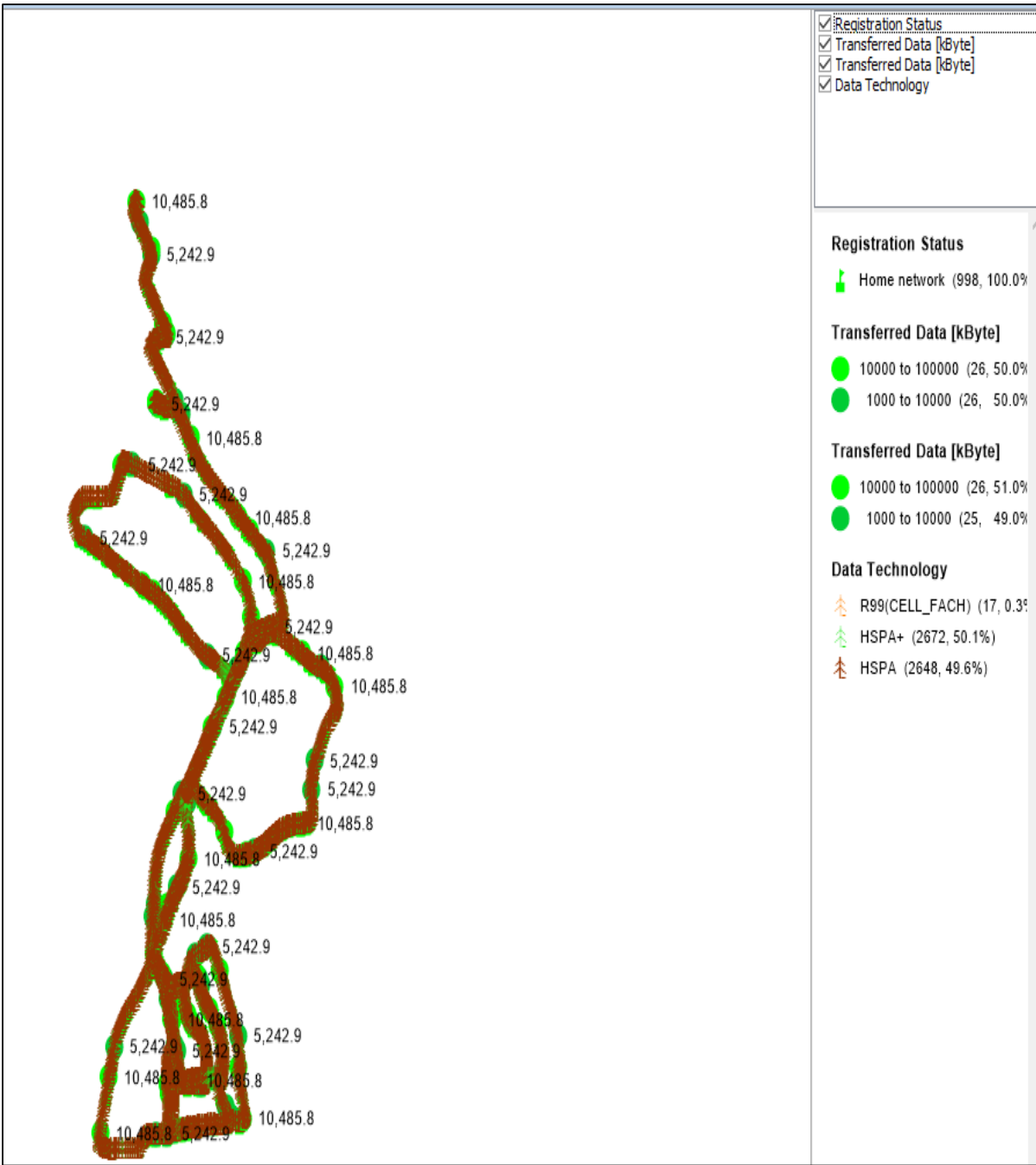
Figure 6: Map of Registration Status, Transferred Data (FTP/HTTP) and Data Technology for Bmobile and TashiCell for 3G_1 network (Samdrup Jongkhar)
