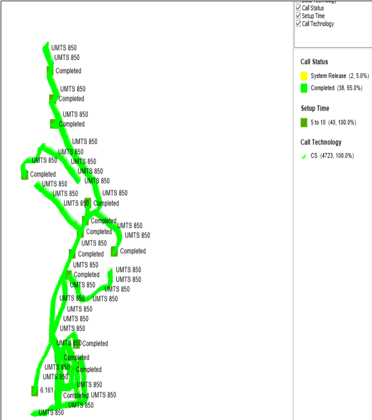
Figure 5: Map of Call Set-Up Time, Call Status and Call Technology of Bmobile and TashiCell for 3G_1 Network (Samdrup Jongkhar)
