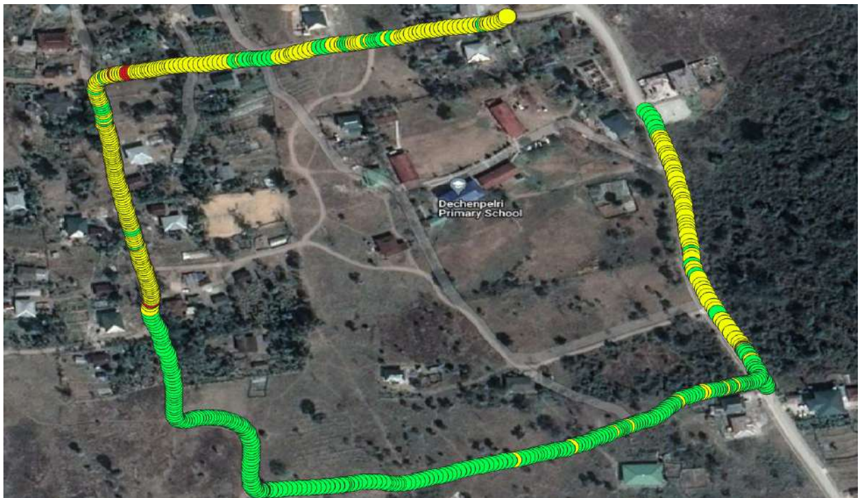
Figure 3.10: RSRP(4G) plot of B-mobile (QGIS) [Dechen Pelri]
