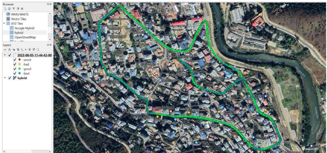
Figure number 1.11: RSRP plot 4G B-mobile (QGIS) [Changzamtog]
