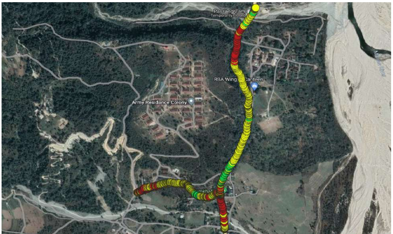
Figure 3.8: RSRP(4G) plot of Tashi Cell (QGIS) [Pelrithang]
