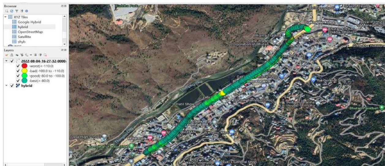
Figure number 1.1: RSCP plot B-mobile (QGIS) [Babesa]
