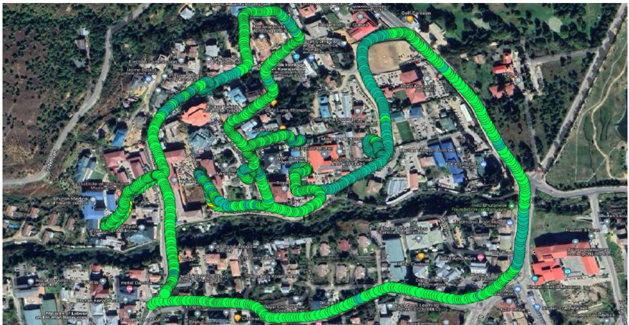
Figure number 1.19: RSRP plot 4G B-mobile (QGIS) - MoIC (including ministry areas, BTL and Kawajangsa)
