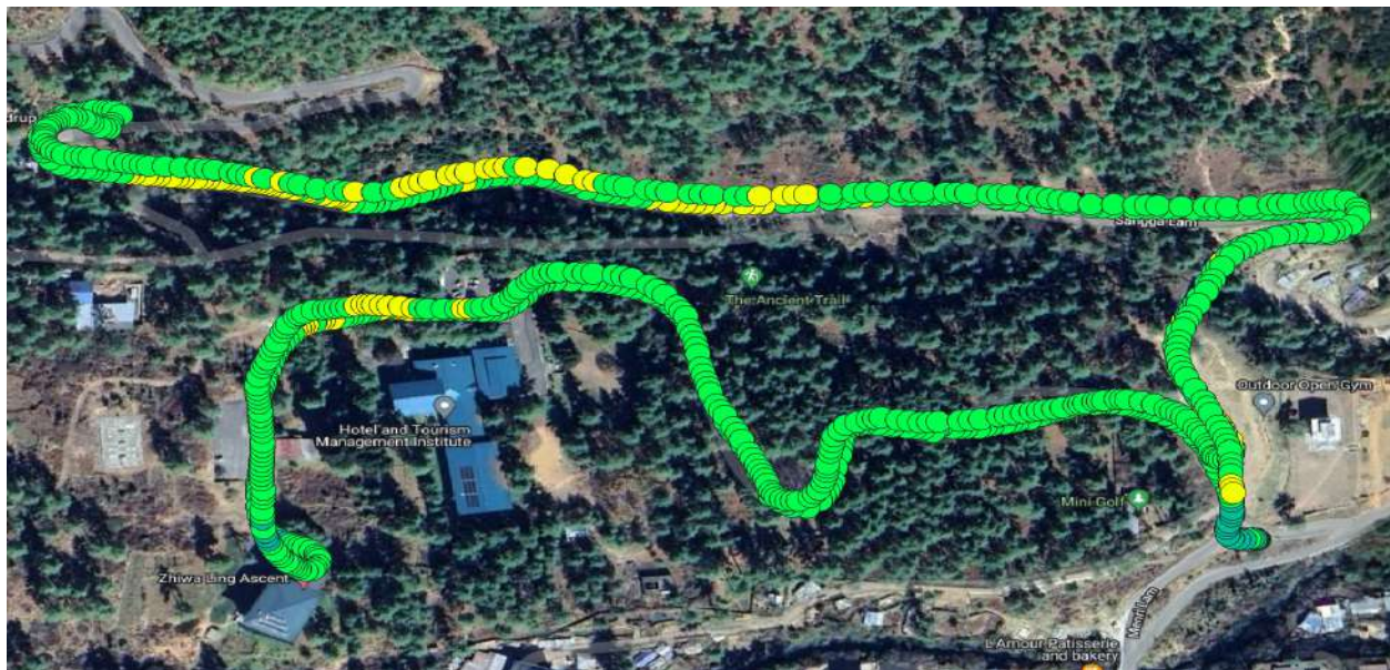
Figure number 1.21: RSRP plot 4G B-mobile (QGIS) - Sangaygang (RITH, Motithang Takin Preserve)
