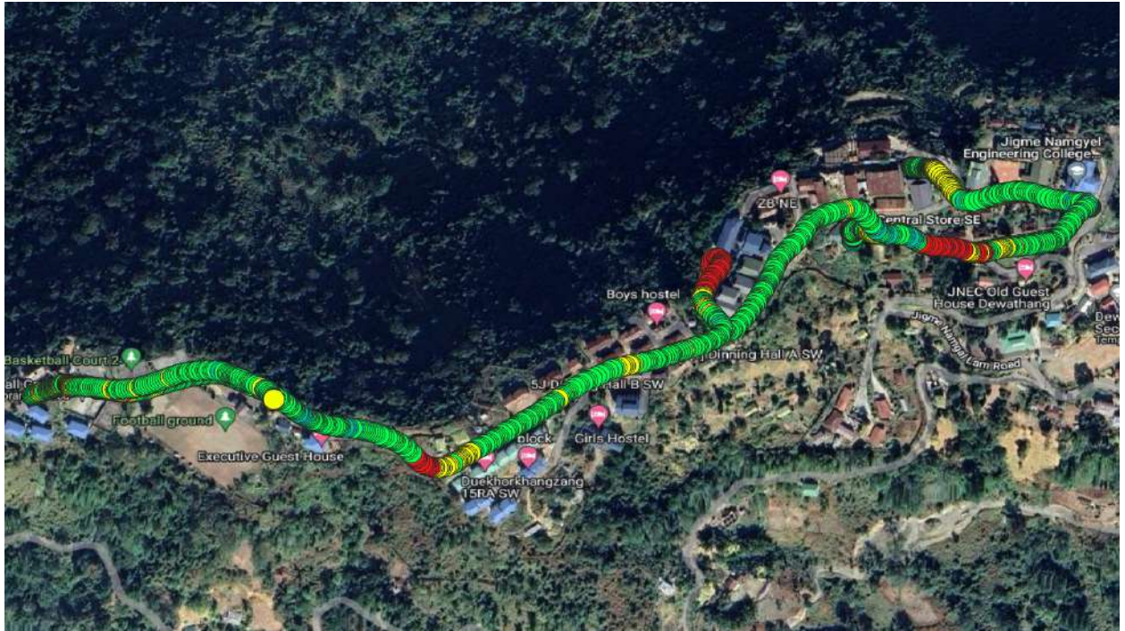
Figure 2.3: RSCP(3G) plot Tashi Cell (QGIS) [JNEC]
