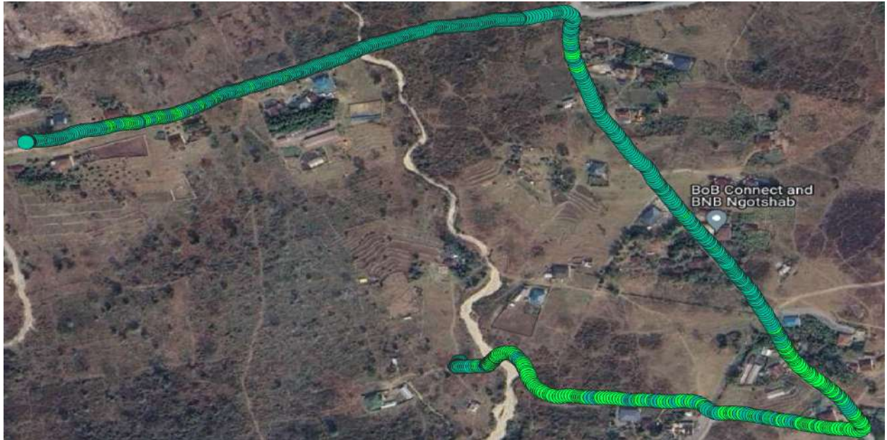
Figure 3.19: RSCP(3G) plot Tashi Cell (QGIS) [Zomlingthang]
