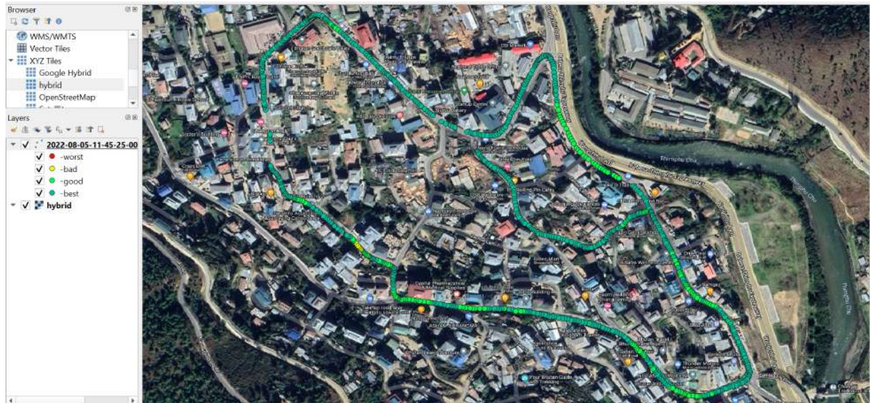
Figure number 1.10: RSCP plot 3G Tashi cell (QGIS) [Changzamtog]
