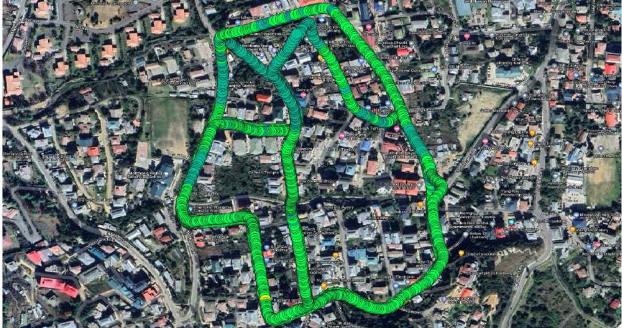
Figure number 1.16: RSRP plot 4G Tashi Cell (Google earth) - Lower Motithang
