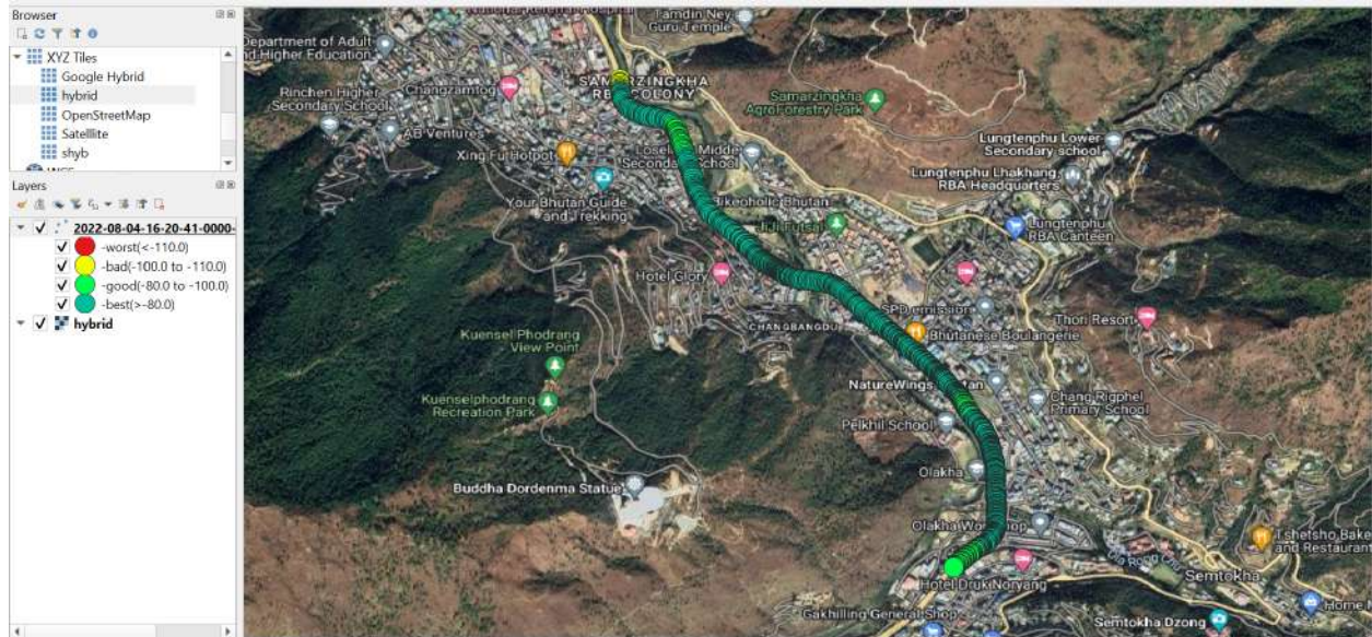
Figure number 1.5: RSCP plot B-mobile (QGIS) [Babesa-Olakha Highway]
