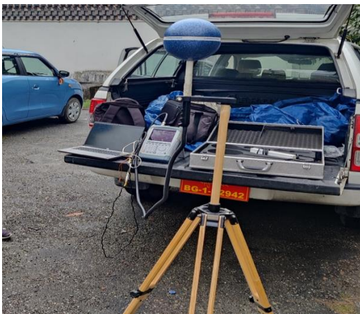
Figure 1: Isotropic Antenna/Type (3-Axis)
