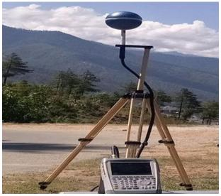
Figure 1: Isotropic Antenna/Type (3-Axis)
