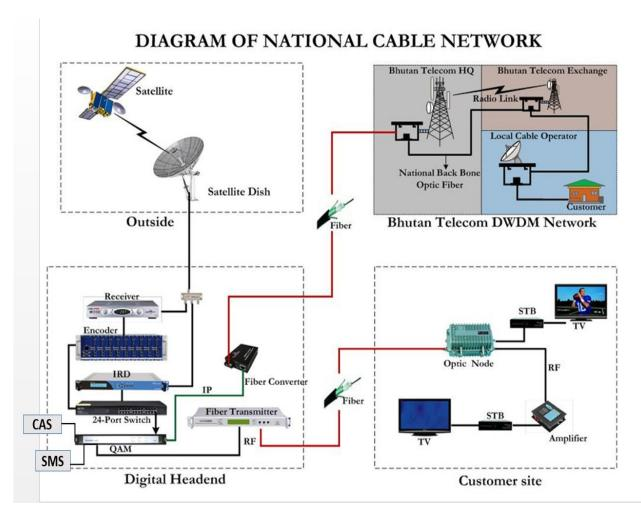
Fig 2: Digital television set up
