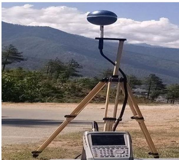
Figure 1: Isotropic Antenna/Type (3-Axis)
