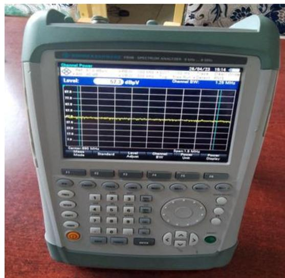
Figure 2: Spectrum Analyzer FSH8
