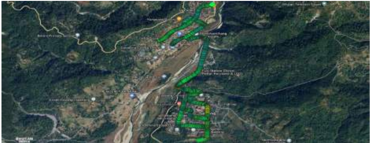
Figure number 5: RSRP plot 4G B-mobile (QGIS) [Sarpang Town and Dzong area]
